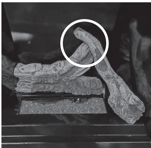
Figure 74: Using a 5/16 drill bit, drill a hole 1in deep in the rear log as shown above. Insert the log pin that was supplied with the unit into the hole.
