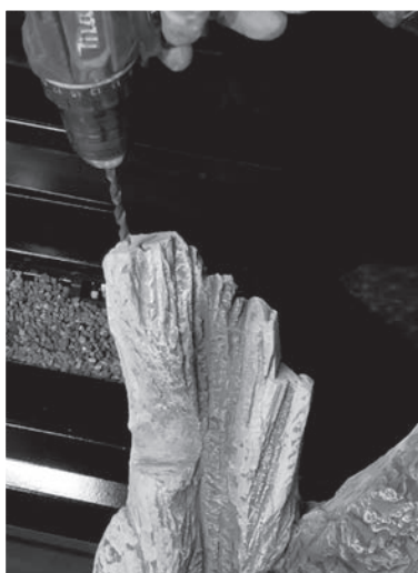
Figure 74: Using a 5/16 drill bit, drill a hole 1in deep in the rear log as shown above. Insert the log pin that was supplied with the unit into the hole.
