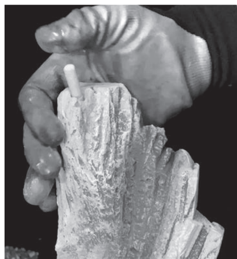
Figure 74: Using a 5/16 drill bit, drill a hole 1in deep in the rear log as shown above. Insert the log pin that was supplied with the unit into the hole.
