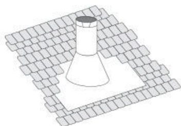
Diagram 11: The upper half of the flashing is installed under the roofing material and not nailed down until the chimney is installed. This allows for small adjustments.
